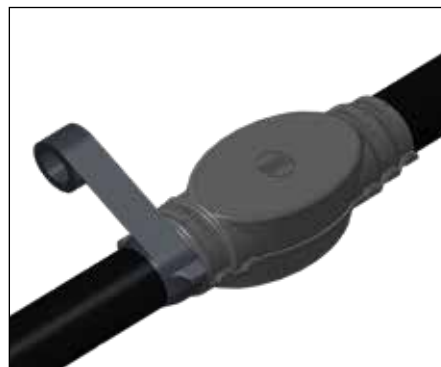
14. Apply self-vulcanizing tape around bundle jacket and work up over FAK ends.
