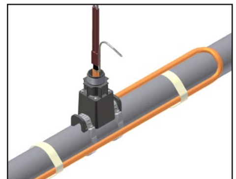
5. Terminate cable with appropriate PETK termination kit. Refer to PETK installation instructions.
