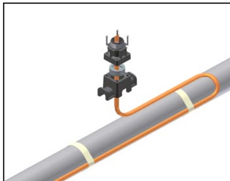
2a. For one, two or three cables. Insert cable into expediter, grommet, and NPT threaded cap.
