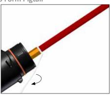
**1c.** Twist braid into a pigtail. Trim ends of braid.
