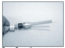
**Power Connection Step 1:** Slide the junction box fitting cap, strain relief disk, grommet, and then gland fitting body onto the power end of cable.
