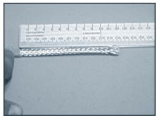
**Step 2:** Cut overjacket back a distance of 5" (120 mm).
