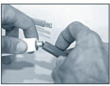
Step 15: Fill the smaller end cap with RTV.
