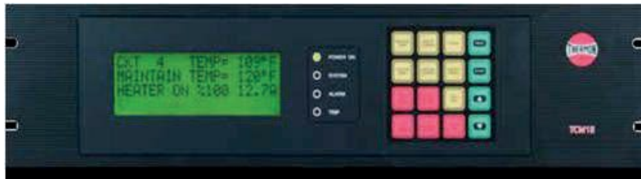
Figure 7: TCM18 Control and Monitoring Module Front Panel
