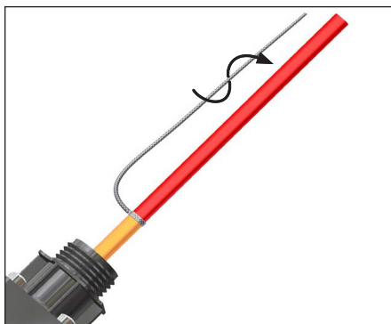
8. Twist braid into a pigtail. Trim ends of braid.
