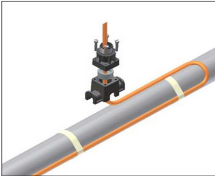
1. For one, two or three trace heaters. Insert trace heater into expediter, grommet, and NPT threaded cap.
