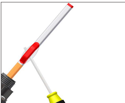
7. Separate braid strands at edge of overjacket and pull trace heater through opening.
