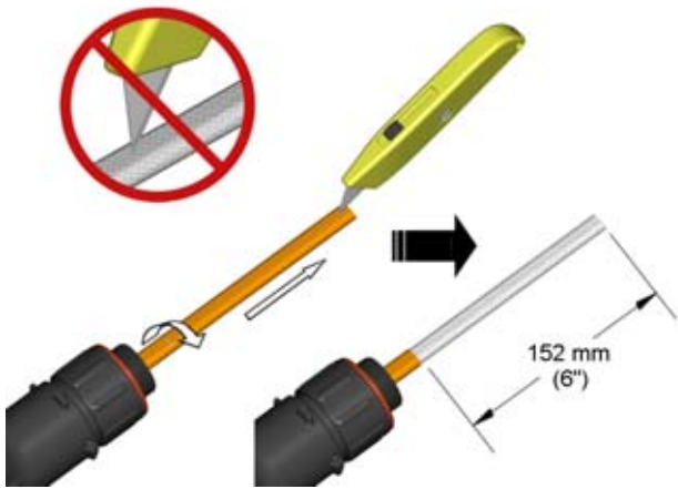
C1. Cut and remove overjacket. Do not cut metallic braid.
