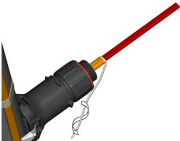
B3. Twist braid into a pigtail. Trim ends of braid.
