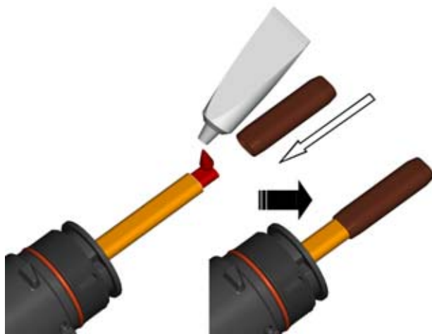
C3. Apply a liberal amount of RTV sealant to cable and slide end cap onto the end of the cable.
