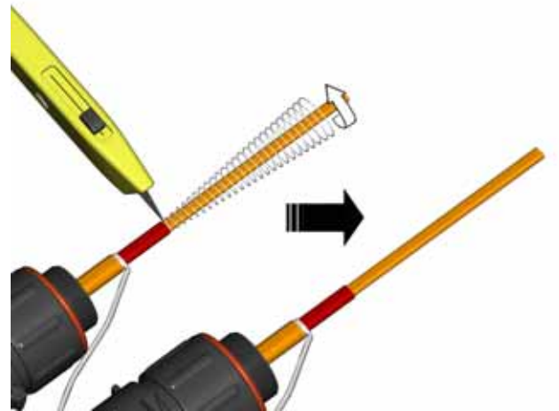
11. Cut and remove heating element and fiberglass overlay (FP cable only). Push any remaining heating element wire under the primary insulation jacket.
