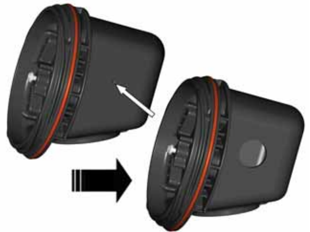
17. Using dimple molded into side of junction box base to locate center of hole, drill for user supplied power connection fittings per manufacturer's recommendations (if necessary).
