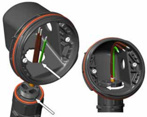
18. Mount junction box base on expediter. Make sure to align slots to properly orient junction box base.
