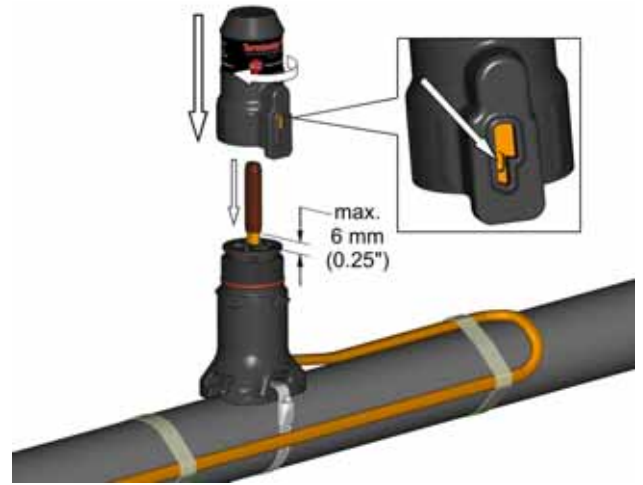
16. Push excess cable back through expediter. Tighten cap securely. Tape cable expansion loop to pipe.
