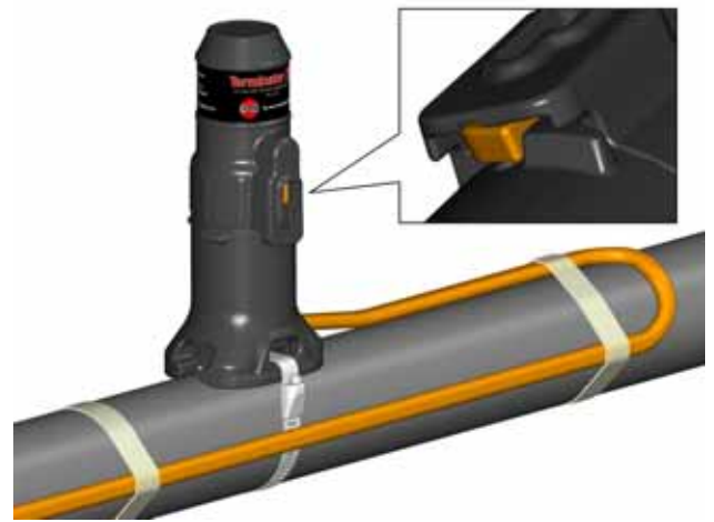
17. Completed end termination kit. Make sure latch mechanism is in the locked position.
