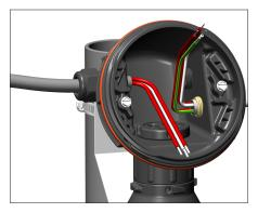
6. Install control wiring (user supplied, 10 AWG [6 mm²] max). 3-wire cable (for 1 sensor) with braided earth shield is recommended.
