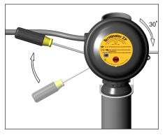
**10.** Use screwdriver to ratchet on junction box lid. Lid will rotate 30 degrees.
