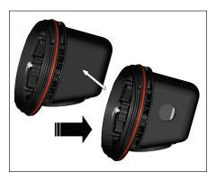
Use dimple molded into side of junction box base to locate center of hole, drill clear M20 hole for sensor gland on one side. On the opposite side drill appropriately sized clear hole for sensor cable gland (customer supplied).
