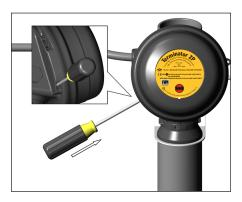
**9.** Install junction box lid and twist hand tight. Insert screwdriver into ratchet slots located on side of junction box base.
