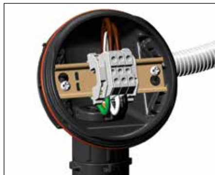
13. Complete system wiring. Refer to typical wiring details. Tightening torque 1.5 Nm–1.8 Nm (1.1 ft-lb–1.3 ft-lb).
