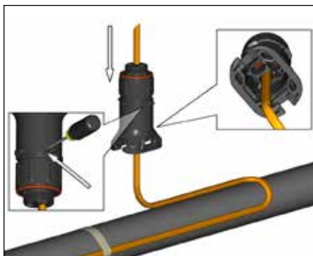
2a. For one, two or three cables. Insert cable into expediter. If mounted on bottom of pipe, punch out weep hole.
