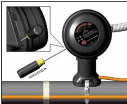
14. Install junction box lid and twist hand tight. Insert screwdriver into ratchet slots located on side of junction box base.
