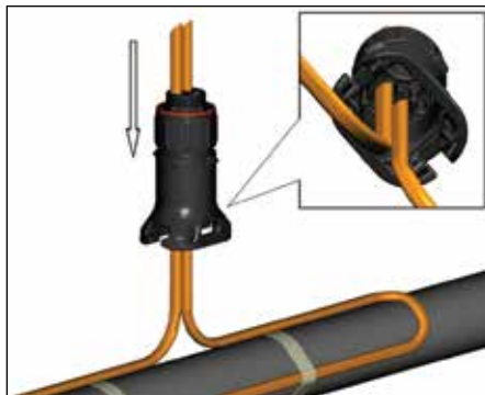
2b. Two cables.
