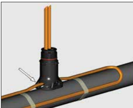
3. Slide expediter toward pipe and route cable through support base entry.
