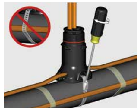
5. Mount expediter to pipe using pipe band. Do not band over cable.
