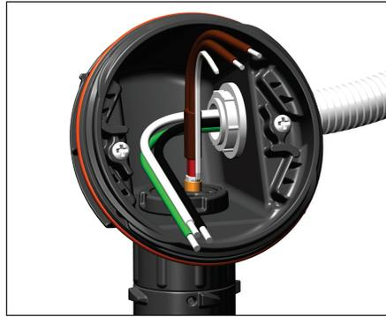
**11.** For power connection applications: Install power connection fittings (user supplied) and pull in power and ground wires.
