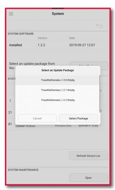
Identify and select the desired firmware package to be installed from the USB.
