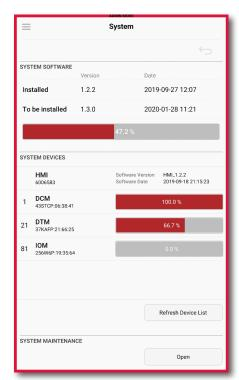
The system will start the installation of the new firmware/software for all Genesis Modules, including the HMI, DCM(s), DTM(s), and IOM(s).
