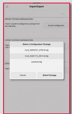
5. Select "Import Configuration" from the Import/Export screen to load a new configuration or restore a configuration from backup.
