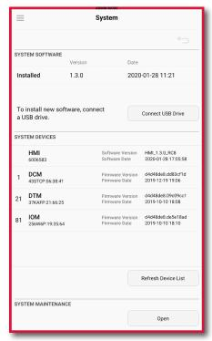
13. The System screen will show the latest firmware installed on each component.
