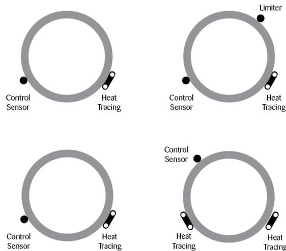
**Figure 16 - RTD Sensor Location**
