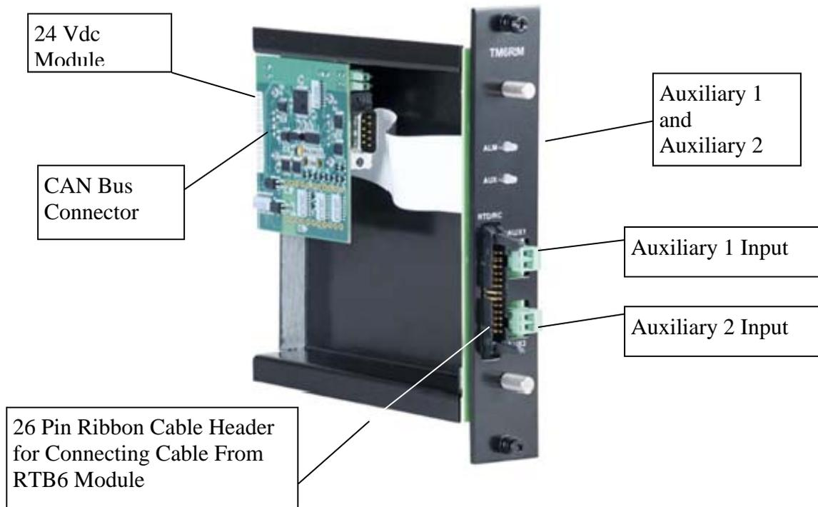
Figure 11 - TM6RM Wiring and Connections
