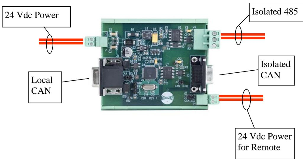
Figure 15- CIM1 Wiring and Connection
