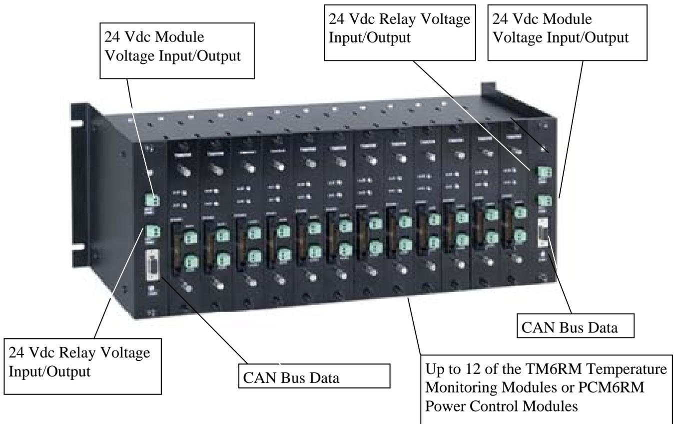
Figure 9 - BPM12 Wiring and Connections
