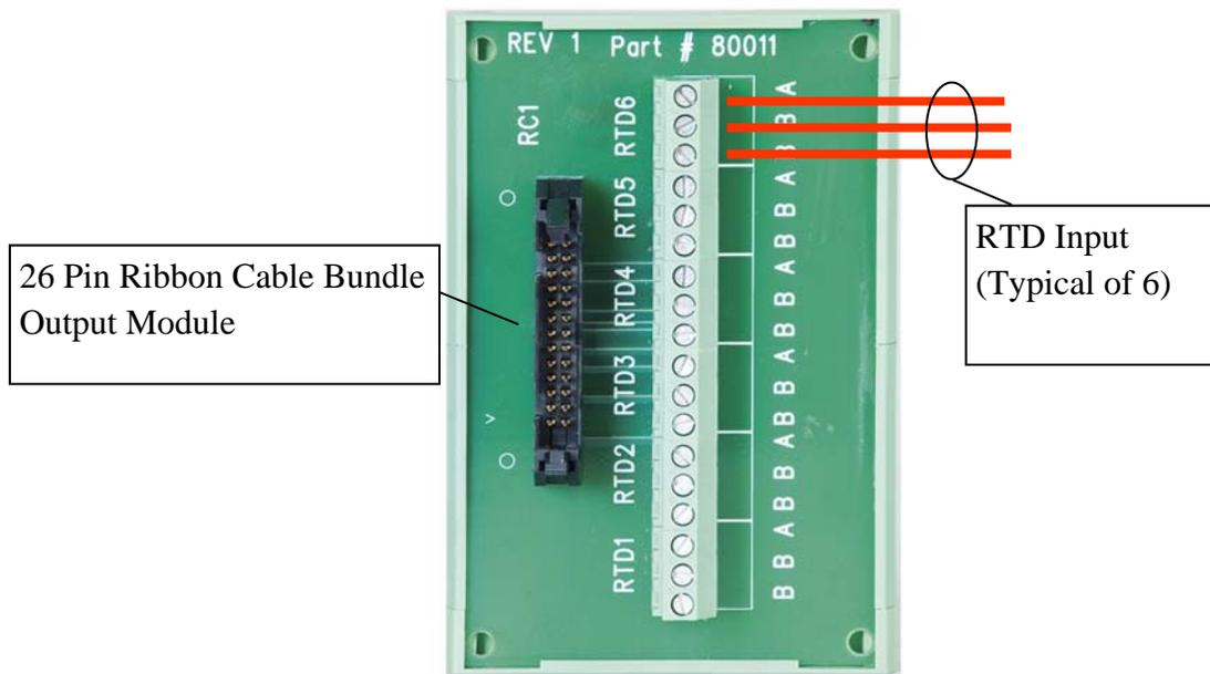
Figure 10 - RTB6 Wiring and Connections
