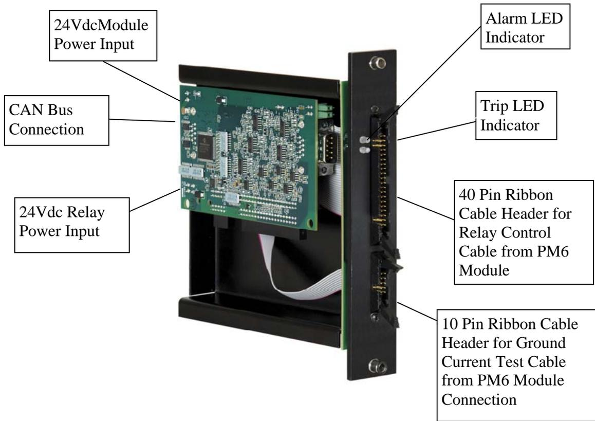
Figure 12 - PCM6RM Wiring and Connections
