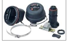
**Terminator DP** is designed to fabricate power connections, in-line/T-splice connections or for making end terminations. Electrical connections are made in terminal blocks utilizing nickel-plated copper terminals to ensure corrosion-free electrical integrity. The up front positioning of the terminal block permits easy access during termination and for future routine maintenance.
