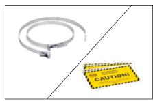
**CL** vinyl-based peel and stick caution labels are intended for direct exposure to industrial environments. Electrically heated pipelines and vessels are to be clearly identified at frequent intervals. Caution labels should be placed at 10<sup>1</sup>-20<sup>1</sup> (3-6 m) intervals or as required by code or specification.
