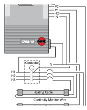
Current Loss Monitoring: The integrity of constant wattage parallel or series heating cables and power-limiting parallel heating cables can be monitored by checking the magnitude of the current in the circuit using the optional CT-60 current sensor. If a 25% loss in current occurs, the CVM-12 will signal an alarm condition.
