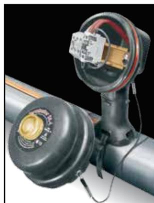
**DS/DE and ZS/ZE<sup>1</sup>** Kit is designed to fabricate accessible outside-the-insulation splices or end terminations of Thermon heating cables. (For applications requiring T-splices the Terminator DP or ZP may be used.)
