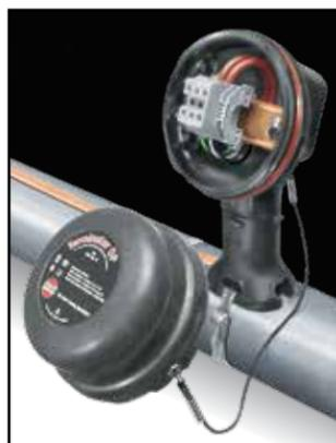
**DL and ZL<sup>1</sup>** End-of-circuit light kit is designed to provide visual indication of an energized heating circuit. The kit may be utilized as an end termination or a power connection. Electrical connections are made in a terminal block utilizing nickel-plated copper terminals to ensure the electrical integrity of the connection over time.
