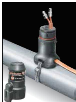
**DE-B and ZE-B<sup>1</sup>** End-of-circuit light kit is designed to provide visual indication of an energized heating circuit. The Standard Terminator Beacon utilizes a high intensity green LED assembly for superior day or night visibility. This light is also available with high intensity red LED.
