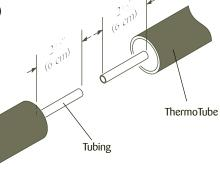
3. Wrap glass fiber tape until level with ThermoTube insulation. Wrap heat reflective tape over fiber tape (25% overlap).
