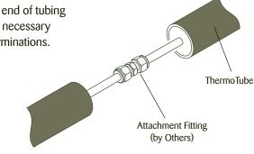
4. Wrap rubber tape around splice forming watertight seal. Allow self-sealing rubber tape to overlap ThermoTube a minimum of 1" (2.5 cm) on each side of splice.
