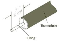
3. Liberally apply RTV sealant to end of ThermoTube insulation.
