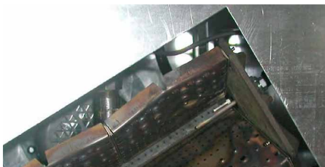
Figure 6 – Flame Rod and Spark Removal
