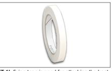
FT-1L fixing tape is used for attaching the heat trace to piping every 30 cm (12") or as required by code or specification. FT-1L may also by used for attaching pipe mounted expediters in circuit fabrication and splice kits. Tape is 13 mm (1/2") wide x 33 m (108') long.
