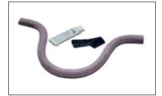
KSR-EJK... expansion joint kits are designed to allow cable to cross a concrete expansion or construction joint. When installed, the kit will allow normal expansion and contraction of the substrate without straining or damaging the heating circuit. Easy-to-use kit includes a reinforced flexible sleeve and RTV adhesive.
