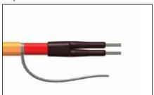
KSR-CFK...circuit fabrication kit for use in hazardous and industrial areas. Terminates SX heating cables in a suitably rated and certified junction box. Kit includes a power boot, end cap, RTV adhesive, and yellow/green earth wire sleeve.
