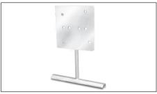
XP-1-140x140 predrilled stainless steel (type 304) mounting bracket designed for mounting Thermon junction boxes directly to the pipe work. The bracket is easily secured to the pipe using B4, B-10 or B-21 attachment bands. The XP-1 is predrilled for use with JB-K-1 and JB-K-2, has plate dimensions of 140 x 140 mm and utilises a 110 mm standoff.
