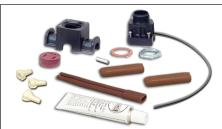
**PCA-COM** circuit fabrication kit is designed to fabricate an HLX circuit with one power connection boot and one end cap. Up to three HLX heat tracers can enter a junction box supported by a PCA-COM kit when additional connection boots (TBX-3L) and end caps (ET-6) are used.
