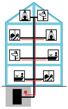
Self-regulating cables are simply taped to the supply piping and insulated. The cable can be cut to length and terminated on site without the need for special tools.
