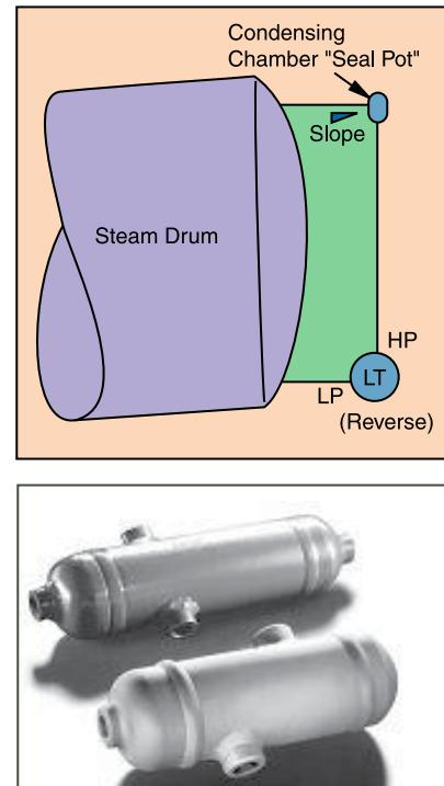
the steam drum. Steam condenses in the chamber or seal pot and fills the impulse line with condensate. The seal pot is located to allow the condensate to drain back to the source thus keeping the liquid level constant.
