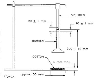
The "V" ratings indicate the material was tested in a vertical position. V-0, V-1, and V-2 indicate that the material self-extinguished within a specified time period after the flame was removed and whether the test specimen dripped flaming particles that ignited a cotton indicator below the sample. VTM ratings are derived from tests designed for very thin materials. 5V ratings are the result of the most severe tests where the flame was applied 5 times.
