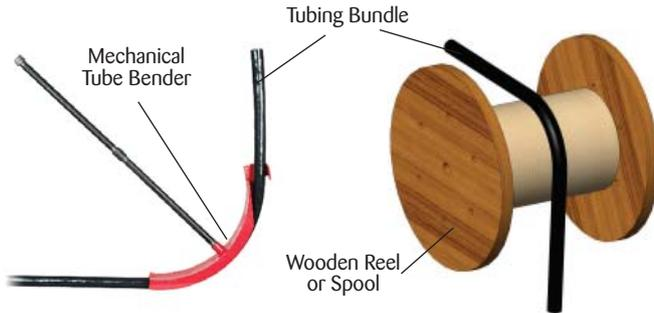
**The Cross-Sectional Area of TubeTrace Tubing Bundle Should Not Be Flattened, Kinked or Wrinkled.**
