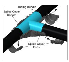
**6.** Cut top and bottom splice cover ends to match outside diameter of tubing bundle.
