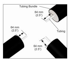
Remove outer jacket and insulation from tubing bundle approximately 64 mm (2.5") from the end of the tubing bundle.
