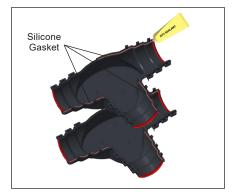
Install silicone gasket, cutting off excess. Apply RTV sealant to both halves.
