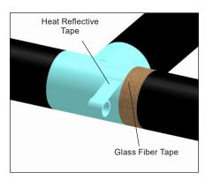
**10.** Wrap with 1 pass of heat reflective tape (50% overlap).
