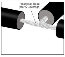
**4.** Wrap high temperature tubing with 1/2" fiberglass rope.
