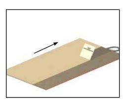
Smooth out adhesive ridges with the spreader. The final adhesive thickness should not exceed 1/32" (0.8mm).
