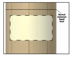
Position heater against tank wall exactly where it is to be mounted. With the marking pen trace the outline of the heater onto the tank wall.
