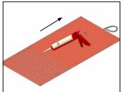
2. Load adhesive tube into caulking gun. Puncture seal and install nozzle. Cut 1/2" (13mm) off of nozzle tip for proper bead size. Apply bead of adhesive around edge of heater, then apply bead of adhesive across heater at 2" (51mm) spacing. In a similar manner apply adhesive to marked area on the tank wall.
