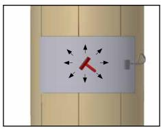
5. Position heater into place within 5 minutes after applying adhesive. Delays will cause the adhesive to "skin over" resulting in heater not bonding to tank wall. Compress heater firmly onto tank wall. Using the roller, work out any air bubbles by running the roller over the backside of the heater from the center outward. The more pressure applied the better the adhesive and heater performance.
