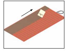
Immediately spread adhesive uniformly on both heater and tank wall using notched edge of Multi use spreader. Be sure entire heater and tank wall area are covered.
