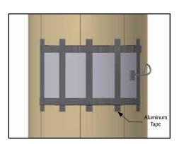
**6.** Secure heater to tank wall as required using aluminum tape. If spray on foam insulation is used seal all edges of heater with the tape to prevent lifting. Allow 24 hours for adhesive to cure before energizing. Secure caution label to exterior of insulation to identify vessel as electrically heat traced.
