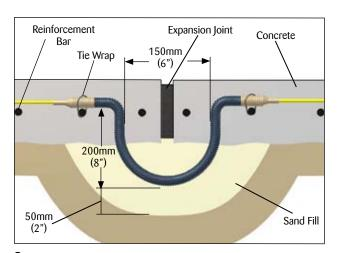
**3.** Typical heating cable layout should be routed to avoid crossing expansion, crack, or construction joints. If crossing a joint is required, the cable and protective tube should be looped beneath the joint, with the cable attached to the concrete reinforcing bar at each end.
