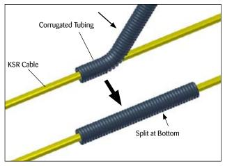
**1.** Insert cable into corrugated tubing through split in tubing. Rotate corrugated tubing until split is facing downward.
