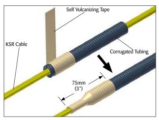
Wrap self vulcanizing tape around heating cable and each end of split corrugated tubing.
