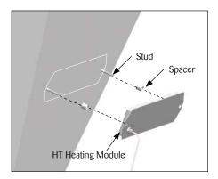
**3.** Place spacer on each stud and then place HT Heating Module over studs.
