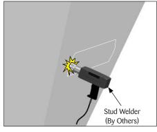
**2.** Weld studs in place per the manufacturer's recommendations.
