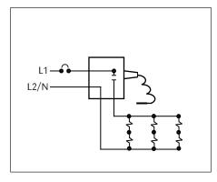
Typical Wiring Schematic for Heating Modules
