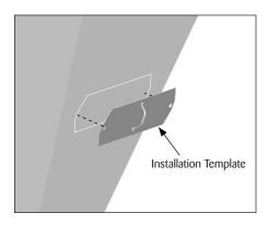
1. Have template and heating system layout drawing available. Select the correct sized template. Position installation template on hopper wall per layout drawing and mark stud locations. If two or more modules are to be placed in one area, care should be taken to insure proper fit of all modules. By marking the outline of each template with chalk or crayon on the hopper wall, clearances can be verified prior to welding of studs.
