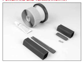
FHT1-F-10 contains components to fabricate 10 power connections and 10 end terminations for FP foundation heating cable. (Components for a single circuit shown.)
