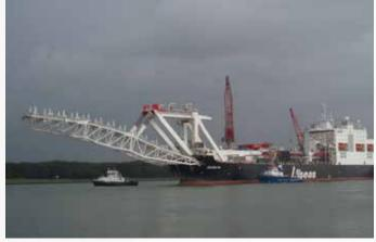
to 7 km per day. The concept of the ship was entirely developed by Allseas, the Dutch company operator of the ship. The length of the ship, excluding the stinger of 106 m, is 225 m and can accommodate a crew of 240. Moreover the ship is equipped with three engine rooms, one for normal propulsion and the other two for powering the six electric thrusters, allowing for exact dynamic positioning.
