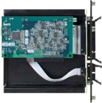
The PCM6RM communicates to both the TSM1 and TM6RM/TM6DR modules through the CAN bus data link.
