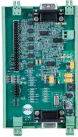
The PCM6DR communicates to both the TSM1 and TM6RM/TM6DR modules through the CAN bus data link.
