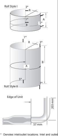
Denotes inlet/outlet locations. Inlet and outlet tubes must be located on opposite diagonals only. (Example: inlet/outlet 1 & 7 or 3 & 5)
