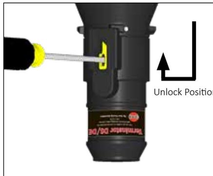
**16.** To remove splice cap, lift latch mechanism to unlock position (as shown) and unscrew.
