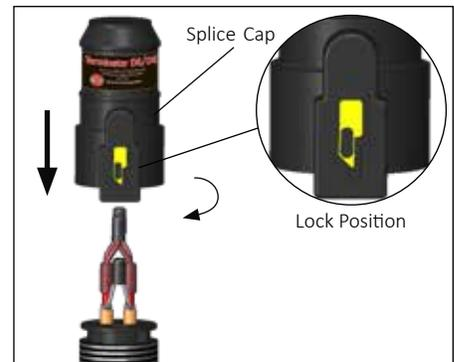
**14.** Mount splice cap to Terminator base, tighten securely. Make sure latch mechanism is in the locked position.
