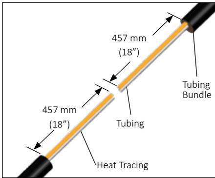
1. Remove outer jacket and insulation from tubing bundle approximately 457 mm (18") from end of the tubing bundle.
