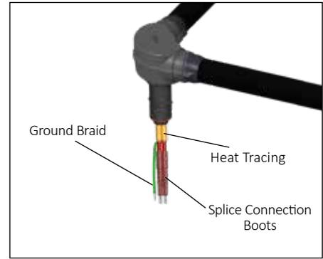
**11.** Terminate heat tracing with appropriate SCTK termination kit. Refer to SCTK installation instructions (purchased separately) for details not addressed here.
