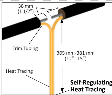
2. Trim tubing to within 38 mm (1-1/2") of the end of the insulation. If self regulating heat trace proceed to step 3. For Zone-type heat trace continue with identification of bus connection on step 2a.
