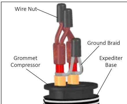
**12.** For splice connections: Connect bus wire using small wire nuts (for BSX, HTSX, KSX) or medium wires. (for RSX, VSX-HT, HPT, and FP). Connect braid wire using large wire nut. See wiring details for splice connections.
