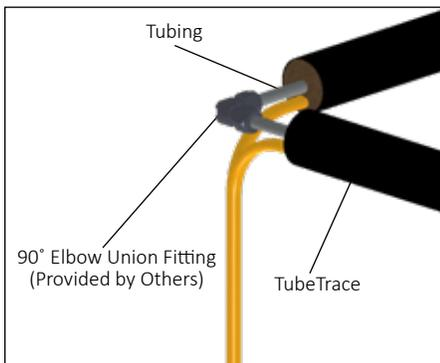
3. Make 90° elbow union connections (fitting provided by others). Test fitting for leaks before proceeding.
