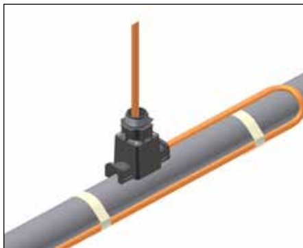
3. Slide expediter toward pipe and route cable through base, grommet, and NPT threaded cap.
