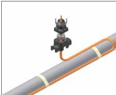
2a. For one, two or three cables. Insert cable into expediter, grommet, and NPT threaded cap.
