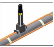
7. Install splice cap using 4 captive screws.
