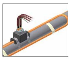
**5.** Terminate cable with appropriate SCTK termination kit(s). Refer to SCTK installation instructions.
