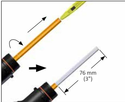
**1a.** Cut and remove heating cable overjacket.
