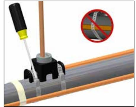
**TracePlus:** Route cable through base entry and mount expediter to pipe using pipe band. **Do not band over cable.**
