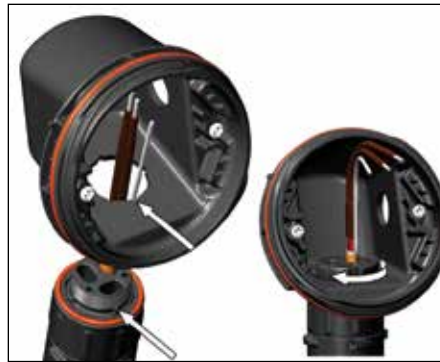
10. Mount junction box base on expediter. Make sure to align slots to properly orient junction box base. Tighten nut securely.
