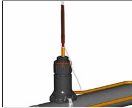
7. Terminate cable with appropriate PETK termination kit. Refer to PETK installation instructions.
