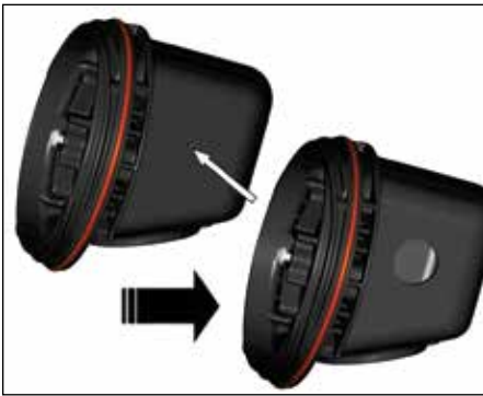
9. For power connection applications: Use dimple molded into side of junction box base to locate center of hole, drill for user supplied power connection fittings per manufacturer's recommendations.
