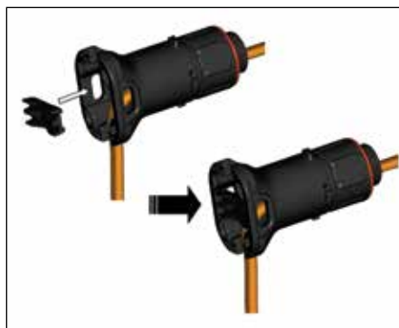
4. Insert banding guide into expediter and snap into place.
