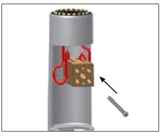
10. Use the terminal block mounting screw to mount terminal block to the LED light module. Bend each pigtail lead around the sides of the terminal block.
