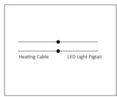
Wiring Schematic for LED Light
