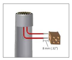
**9.** When using SCTK-TB Connection Kit, first trim exposed bus wires of the LED pigtail to 8 mm (.32"), then connect to the terminal block.
