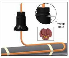
**2.** Insert cable into expediter. If mounted on bottom of pipe, punch out weep hole.
