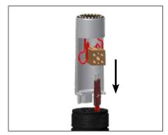
**11.** Connect the bus wires of the trace heater to the terminal block.
