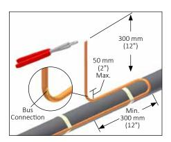
Locate bus connection (HPT and FP only) and cable as shown. Cut end of cable at angle to aid in piercing grommet. Leave additional cable for expansion loop.
