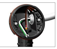
**11.** For power connection applications: Install power connection fittings (user supplied) and pull in power and ground wires.
