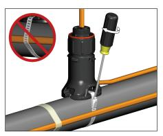
**5.** Mount expediter to pipe using pipe band. Do not band over cable.
