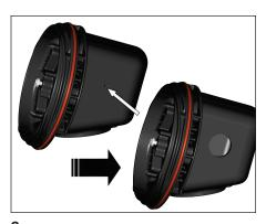
**9.** For power connection applications: Use dimple molded into side of junction box base to locate center of hole, drill for user supplied power connection fittings per manufacturer's recommendations.
