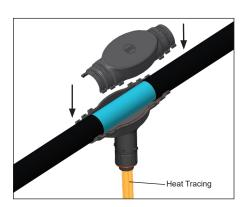
12. Assemble splice cover top, tubing bundle, and splice cover base together as shown. Snap together firmly. Inspect ends of tubing splice cover for snug fit. Apply additional RTV sealant where needed.
