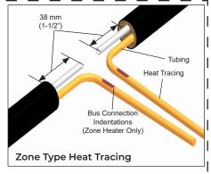
2a. Strip back bundle insulation 38 mm (1-1/2") beyond bus connection indentation of each heat tracing. If bus connection indentation is less than 305 mm (12")-381 mm (15") from end of the heat tracing, proceed stripping the bundle insulation to the next indentation. Trim tubes so the bus connection indentation on each meet.
