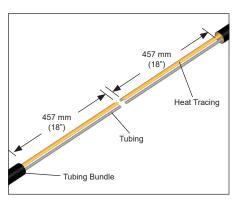
Remove outer jacket and insulation from tubing bundle approximately 508 mm (20") from end of the tubing bundle.
