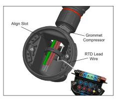
17. Mount junction box on expediter making sure to align slots to properly orient junction box base. Tighten nut.
