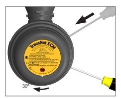
21. Install junction box lid and twist hand tight. Insert screwdriver into ratchet slot located on side of junction box base to tighten. Use screwdriver ratchet on junction box lid. Lid will rotate 30°. To remove lid, repeat steps but in opposite direction.
