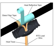
**10.** Complete with additional passes of heat reflective tape.
