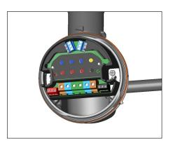
18. Install ECM electronic control module and complete system wiring. Terminal set screws shall be tightened to a torque value of 1,4 Nm (12,4 lb-in). See wiring details. Set ECM modules electronic control and/or control limiter at desired setpoints.
