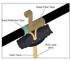
9. Wrap tube and heat trace with 1 pass of reflective tape (25% overlap), then wrap with 3 passes of glass fiber tape (50% overlap), or until fiber tape is equal to original bundle insulation thickness.
