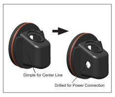
16. Locate the dimple molded into side of junction box base, identify center hole, drill for user supplied power connection fitting per manufacturer's recommendations.
