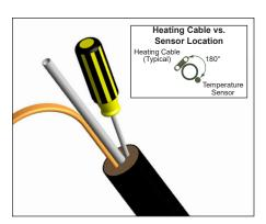
With a screw driver, create a gap for the sensor between the insulation and the tubes and place the sensor inside.
