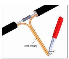
Cut the ends of the cable at an angle to aid in piercing grommet.
