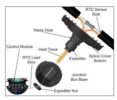
Route RTD tip through expediter nut and expediter opening in junction box base. If necessary, apply lubricant (user supplied) to the end of RTD tip. Slide through conical grommet hole. Insert the tracing cables through conical grommet holes and punch out weep hole.
