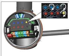
19. Use the rotary switches for settling Control and Limit Temperature, (Celsius or Fahrenheit) and Auto or Manual reset (Control switches on Type "C" or "CH" and both on Type "CL"). Refer to ECM user manual for further details.
