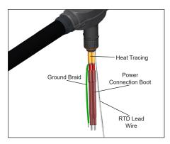
**15.** Terminate heat tracing with appropriate PETK termination kit. Refer to PETK installation instructions (purchase separately) for details not addressed here.
