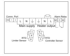
20. Wiring Details: Connection (for Heat Trace, RTD Sensor Leads, Alarm and/or Communication Connections)
