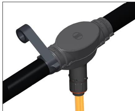
13. Apply self-vulcanizing tape around bundle jacket and work up over FAK ends.
