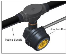
22. Completed TraceNet ECM / FAK-4(L) In-Line Power/Splice Kit for TubeTrace Type SE/ME Bundle (Installation shown is to feed power in the middle of a TubeTrace bundle. Many installations will be near the end of a TubeTrace bundle.) Install bundle clamps (order separately) 300 mm (12") before and after In-line power kit.
