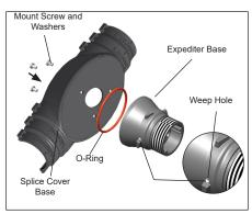
Mount expediter base with o-ring to the splice cover base using (3) M5 mounting screws and lock washers. Punch out weep hole.
