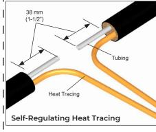
Trim tubing to within 38 mm (1-1/2") of the end of the insulation. If self regulating heat trace proceed to step 3. For Zone-type heat trace continue with identification of bus connection on step
