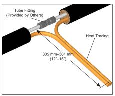
Make tube fitting connections with appropriate fitting (provided by others). Test fitting for leaks before proceeding. Mount tube fitting shifted from each other in case of multiple tubes.
