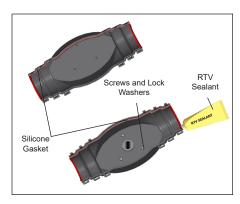
Install silicone gasket and cut off excess. Apply RTV sealant to both halves.
