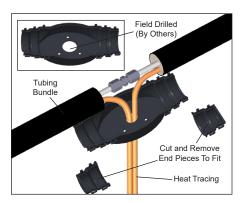
**6.** Cut splice cover ends to match outside diameter of tubing bundle. Field drill expediter base holes.
