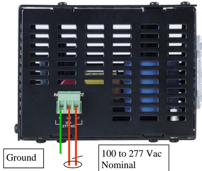
**Figure 4 - Input Power Wiring for the PS70**
