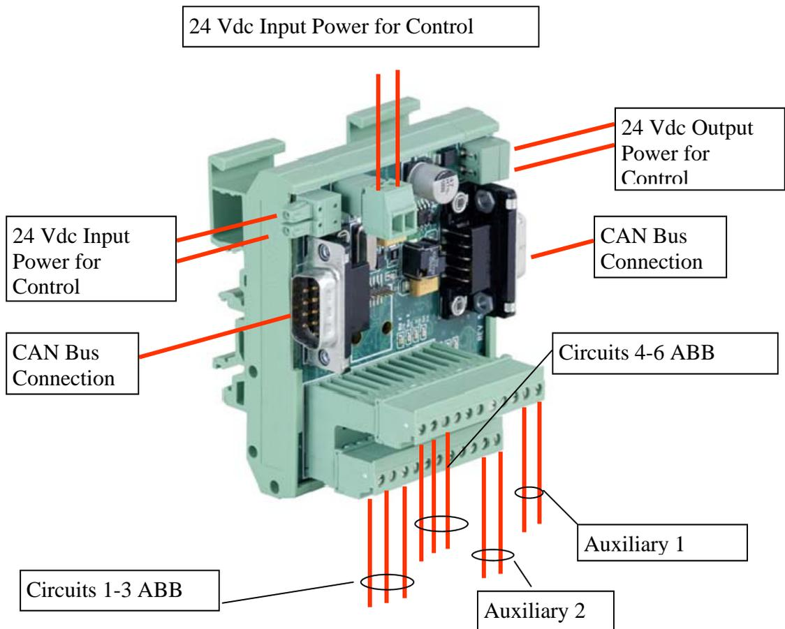
Figure 7 - TM6DR Wiring and Connections
