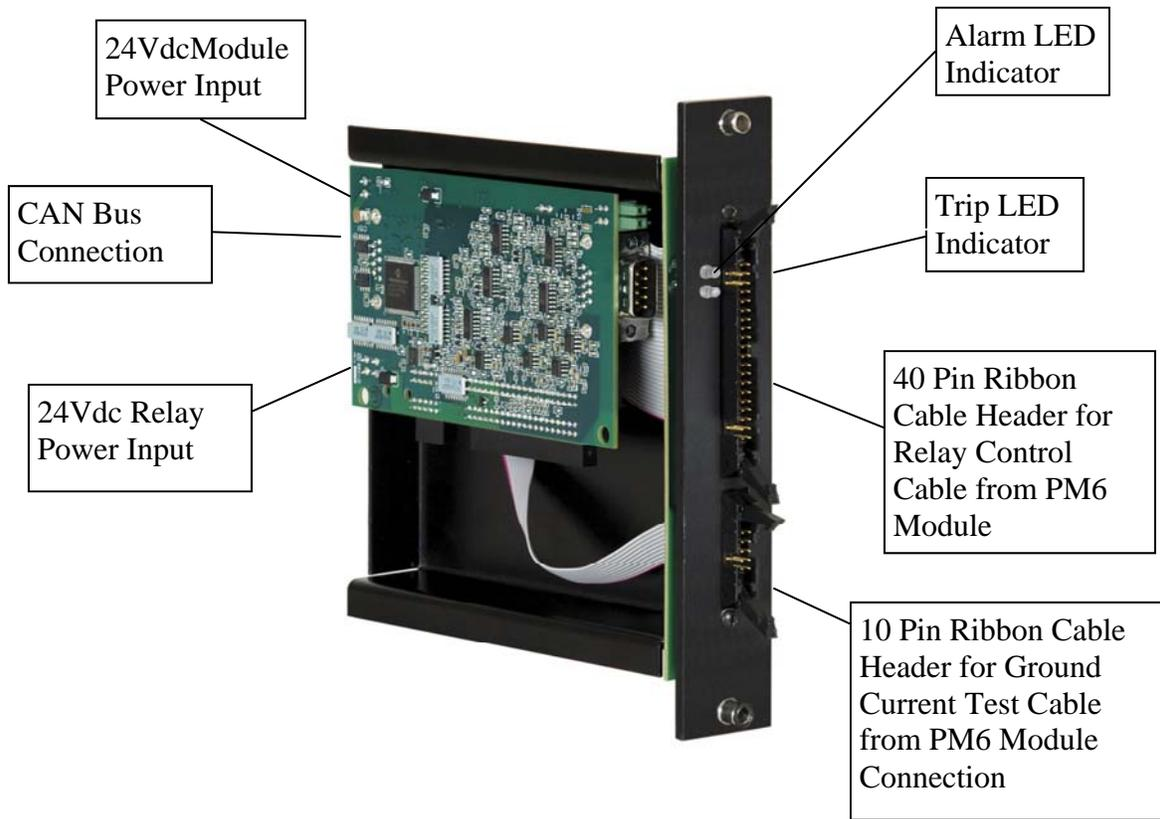
Figure 12 - PCM6RM Wiring and Connections
