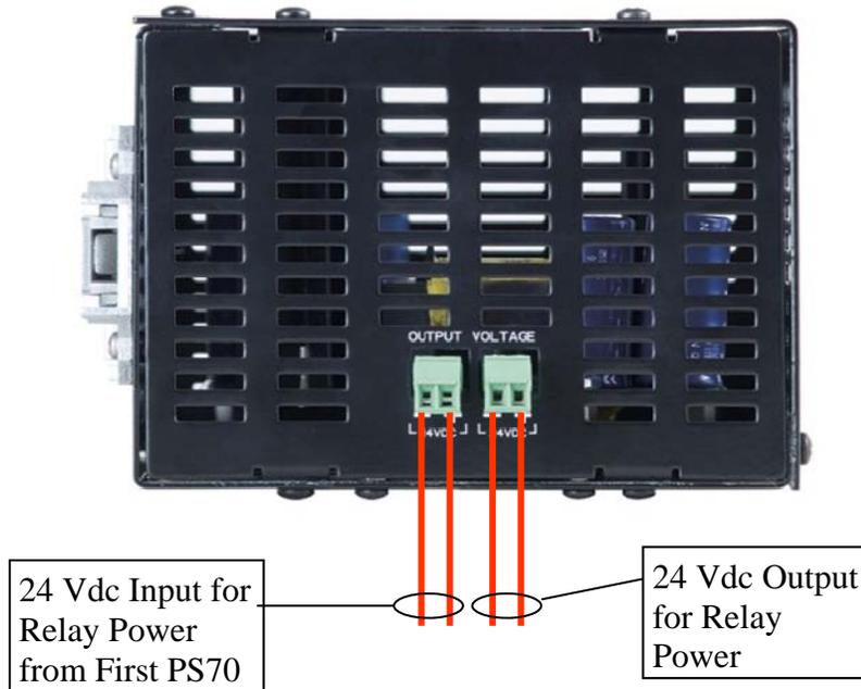
**Figure 3 - Wiring and Connection for Dual PS70**
