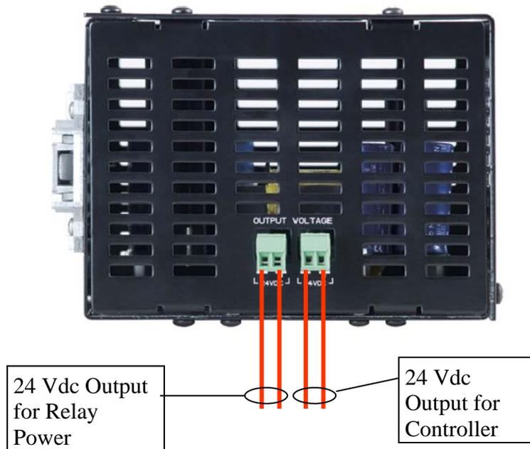
**Figure 2 - Wiring and Connection for Single PS70**
