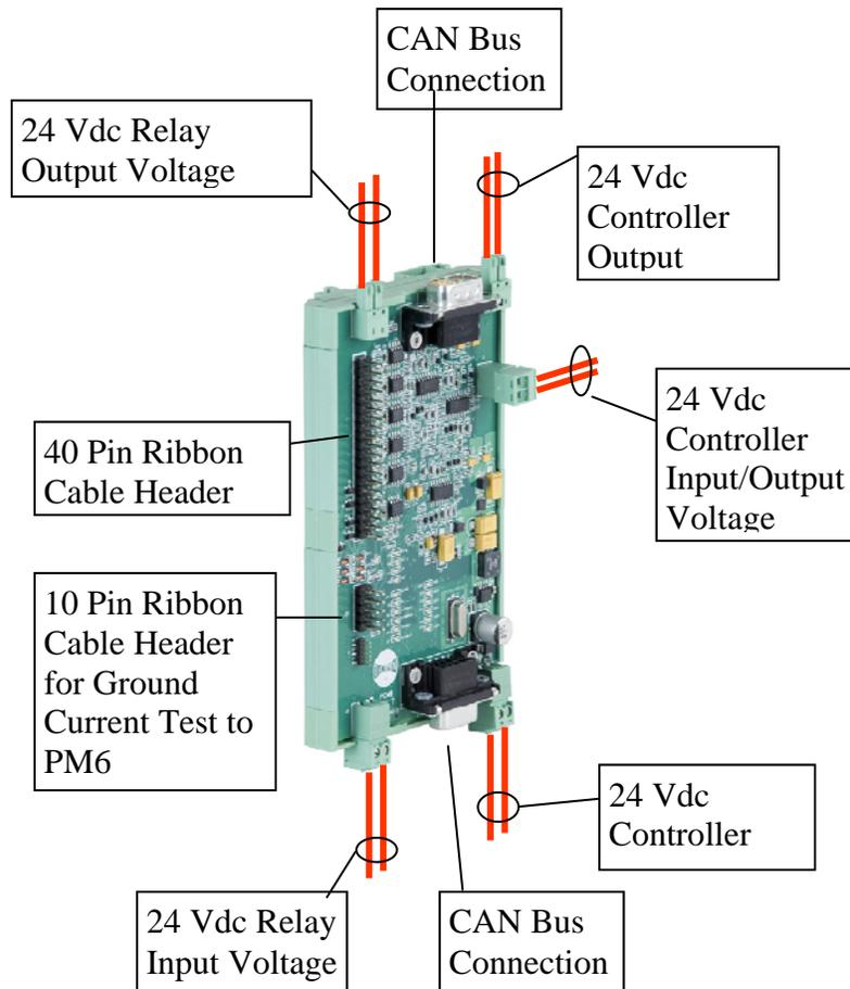
Figure 8 - PCM6DR Wiring and Connections
