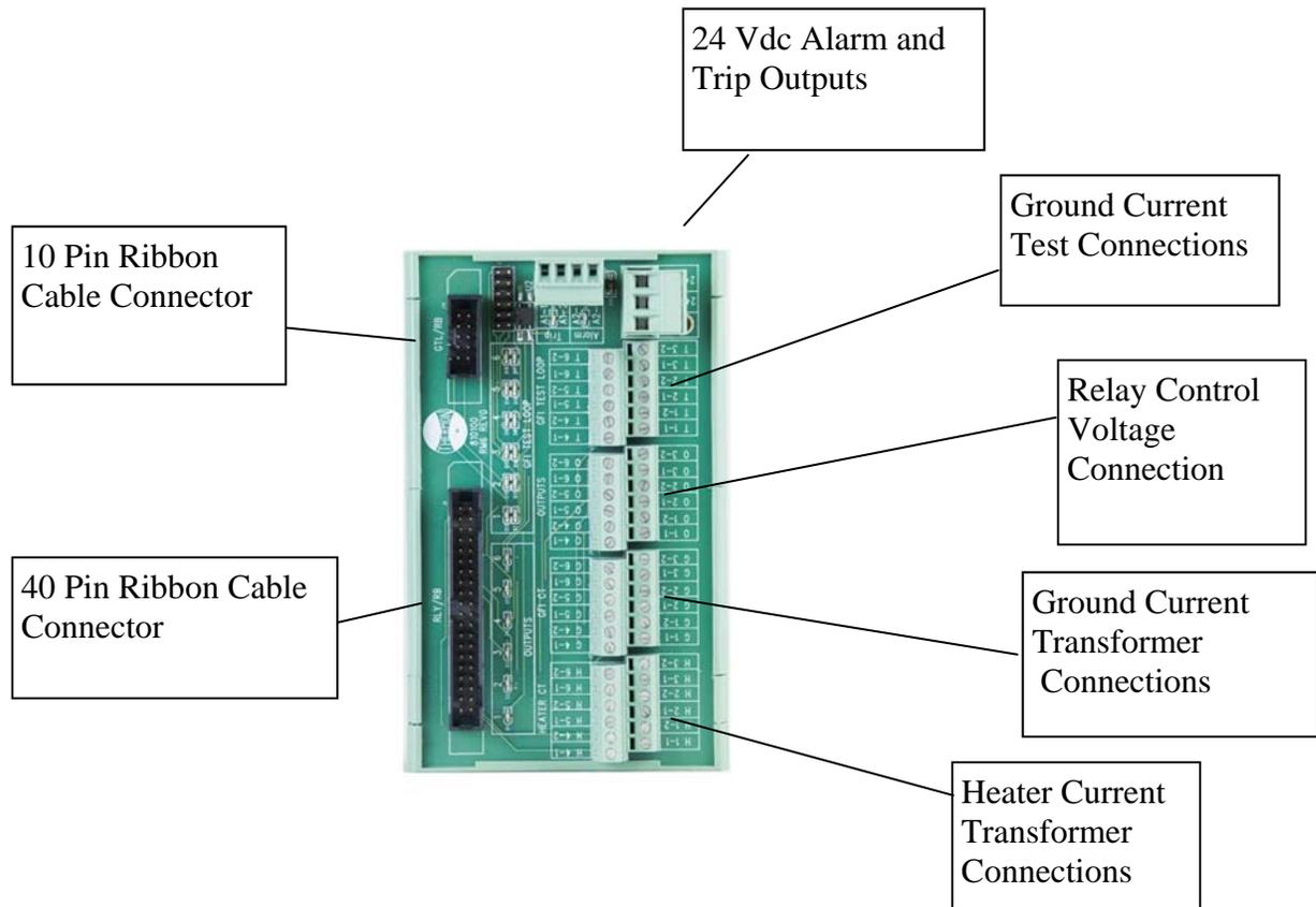
**Figure 14 - RM6 Wiring and Connection**
