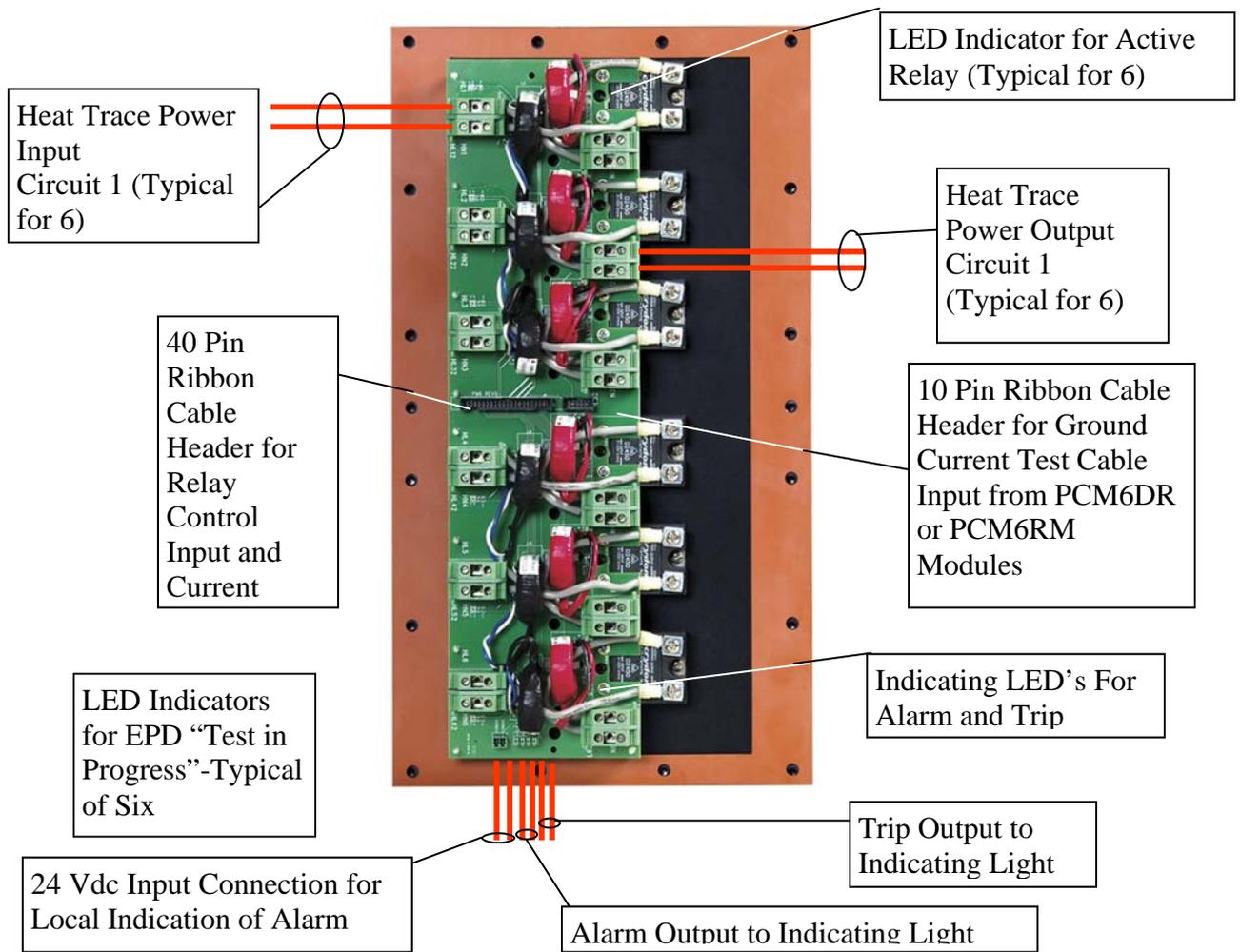
Figure 13 - PM6 Wiring and Connection
