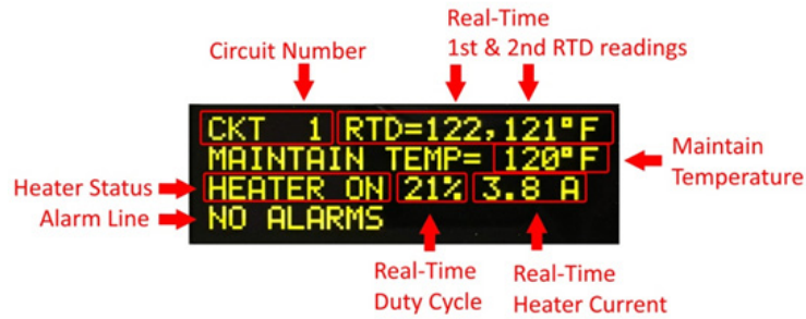
Figure 5.2: Typical Circuit Screen
