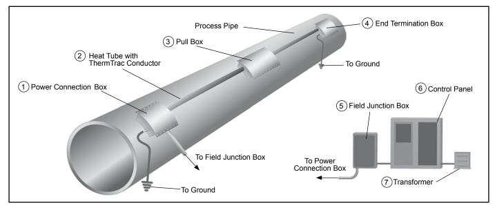
**1. Power Connection Box:** Located at the power feed end of the ThermTrac circuit, the power connection box permits the connections that supply electrical energy to the system. An external tab on the box permits grounding of the system.
