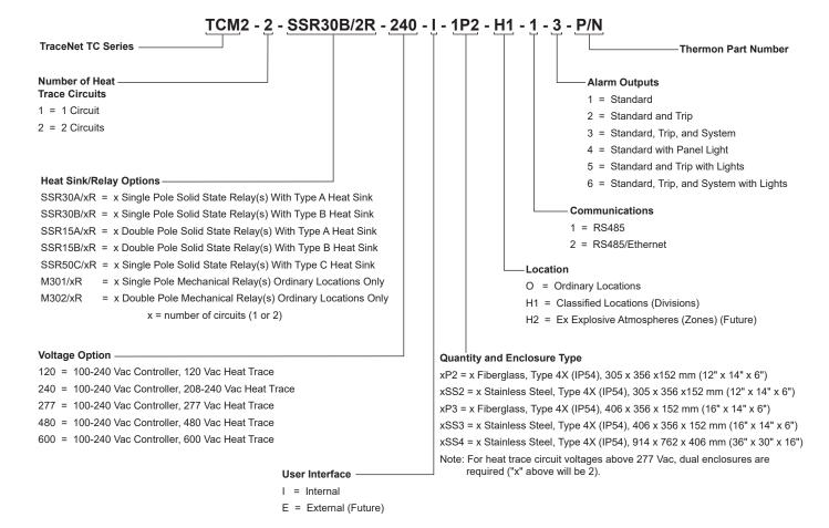
TCM2-FX Control Panel for UL 515A Fire Sprinkler Applications, order the TCM2-FX, with Model Code: TCM2-1-M252/2R-240-I-1P3-O-1-2. This model works for 100-240 Vac controller voltage and 100-277 Vac heat trace voltage.
